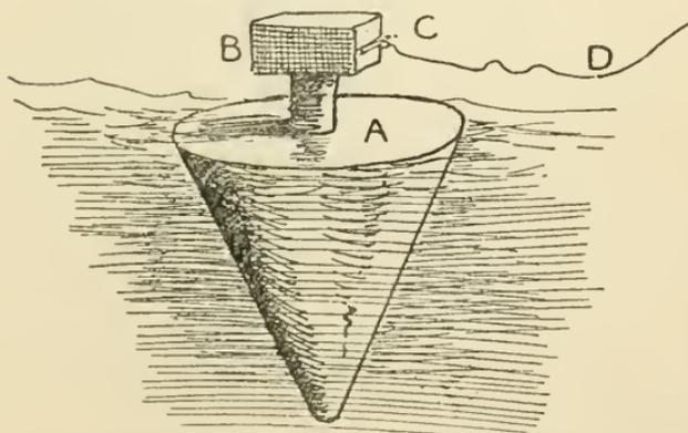
A, Can buoy containing powder. B, Box containing lighted match and punk
